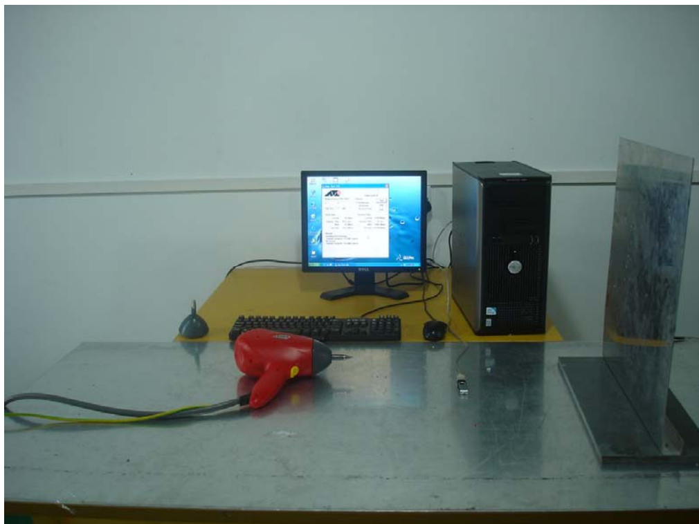
Photo 2 Electrostatic Discharge Test Setup
